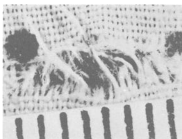
FIG. 5—A hole, in a plain-weave shirt, caused by a stab with the screwdriver. The yarns are long and stretched, with variation in fiber length both within and between yarns. One division = 1 mm.
